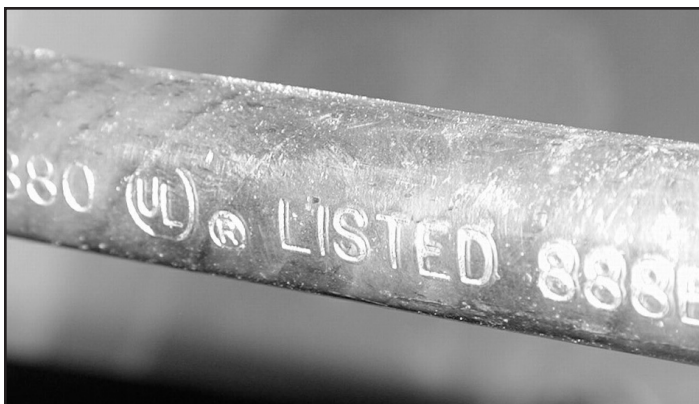
Figure 2 — UL Label Etched into Rod
